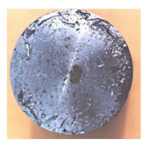
flushed to remove any remaining debris that could cause the same problem. If the cause was big end failure then the crank must be replaced along with the main bearings and seals.
