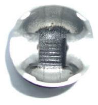
Symptom - Underside of the piston has a dark black spot.
