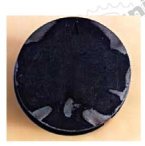
The crown of the piston shows an ideal carbon deposit pattern. The transfer ports on the engine are flowing evenly and the carbon deposits are a dark chocolate brown colour. This indicates that the bike's engine has been set up and jetted correctly.
