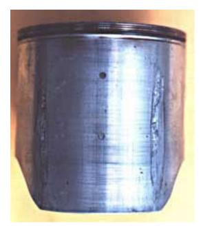
Symptom - The piston has vertical seizure marks at four equally spaced points around the circumference.
