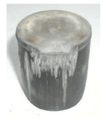
Any engine that is suffering from coolant being forced out of the radiator cap's vent tube suggests a strong indication of a head gasket leak. In most cases the top of the cylinder and the face of the cylinder head must be resurfaced when a leak occurs.
